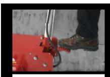
Foot pedal activates quick raise saddle to the lift point available for all long chassis service jacks
